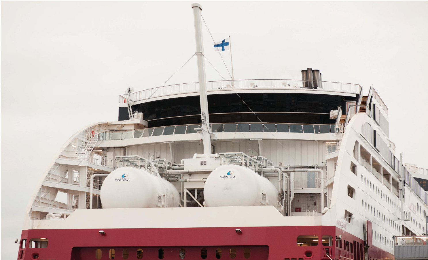
Fig. 3. MS Viking Grace, a cruise ferry powered by liquefied natural gas, has been safely carrying passengers since January 2013.
