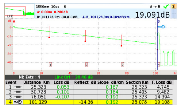
Graphical representation of the fiber optic link, also called an OTDR trace
