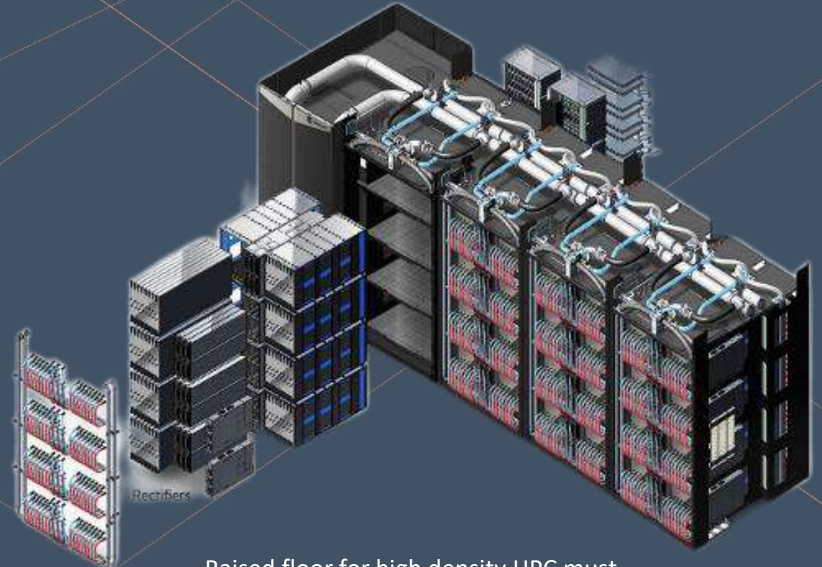
Raised floor for high density HPC must now be ready for 3 tons pr. square meter
