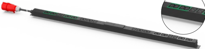
EPI 24+6 3x16A G2 • IN: IEC60309, 3x16A OUT: 24xC13, 6xC19
